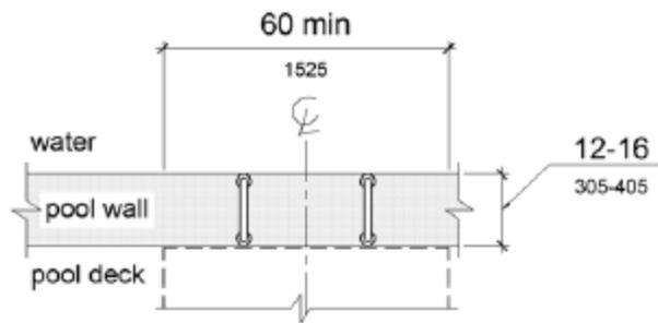
**Figure 1009.4.3 Depth and Length of Transfer Walls**
