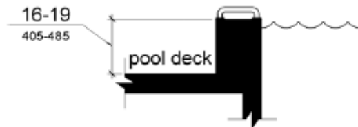
Figure 1009.4.2 Transfer Wall Height
